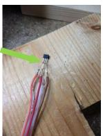
Place the sensor on a flat surface with its curved side down.
