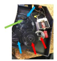
Make a careful note of how the gears are arranged (!!) then remove the two intermediate gears and their shafts (red arrows).
