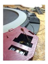
This is the position of the capacitor which allows the plinth to be removed from the base.
