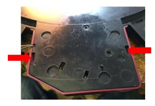
Turn the turntable over, and identify the apertures for the plinth retaining clips.
