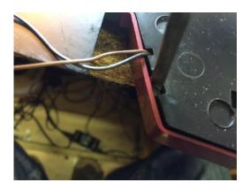
Insert a screwdriver as shown. Carefully twist and then move outwards to ease the side of the plinth away from the base (by a few mm only – do not use excessive force!).
