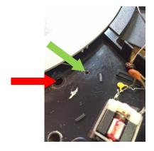
This photograph shows the hole which has been drilled through the base (green arrow).
