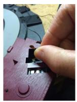
Bend up the leads on the motor suppression capacitor so that the capacitor is clear of the plinth.
