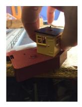
Squeeze the control cabin sides, as shown, to release the clips.
